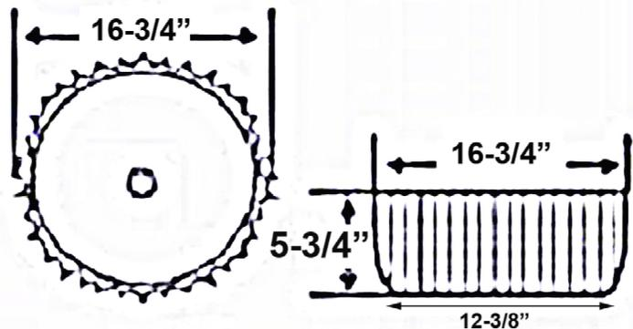
**Dimensions of fixture are nominal and may vary within the range of tolerances established by AMSE Standard A112.19.2.2013 Dimensions and specifications subject to change without notice.**
