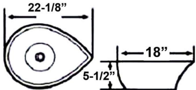
**Dimensions of fixture are nominal and may vary within the range of tolerances established by ANSI Standard A112.19.2.2013 Dimensions and specifications subject to change without notice.**
