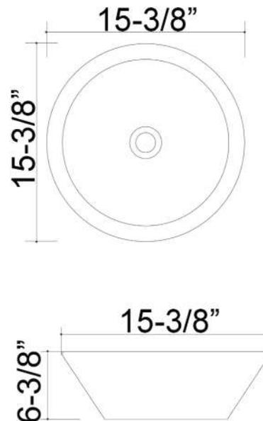
Dimensions of fixture are nominal and may vary within the range of tolerances established by AMSE Standard A112.19.2.2018 Dimensions and specifications subject to change without notice.
