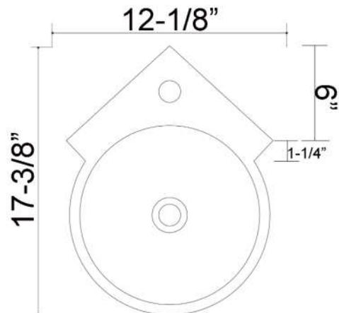
Dimensions of fixture are nominal and may vary within the range of tolerances established by ANSI Standard A112.19.2.2018. Dimensions and specifications subject to change without notice.
