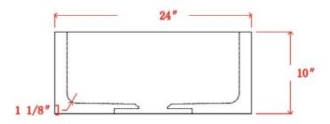
Dimensions of fixture are nominal and may vary within the range of tolerances established by ANSI Standard A112.19.2. Dimensions and specifications subject to change without notice.
