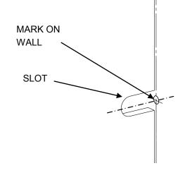
Drill one 3/16" diameter hole approximately 1-1/2" deep at the mark just made. Drill through tile an backer board. Do not drill through blocking.
