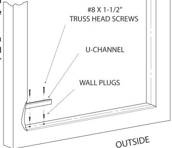
Insert a small amount of silicon into each drilled hole, followed by a wall anchor.
