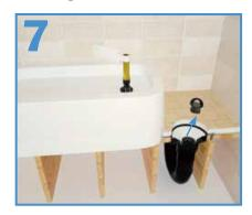
Remove the plug. For easier insertion, apply lubricant to the tailpiece. Be sure to position the bathtub and tailpiece in line with the drain body.
