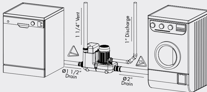
**Powerful 1 HP drain pump meant for commercial applications** where hot water can be an issue as it is capable of handling up to 194°F.
