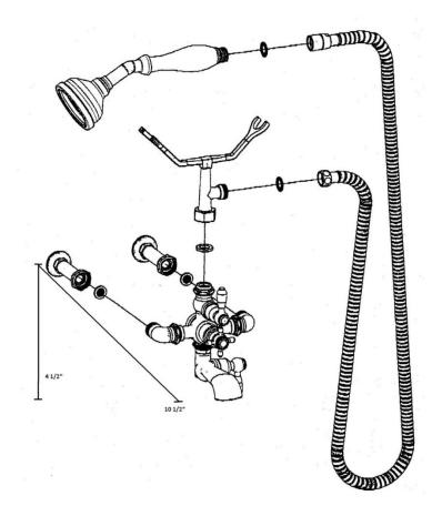
This faucet is tested to remain within 1 degree Fahrenheit of your desired setting throughout its operation, with an automatic temperature stop at 104 degrees Fahrenheit. The unit also has a built-in anti-syphon.
